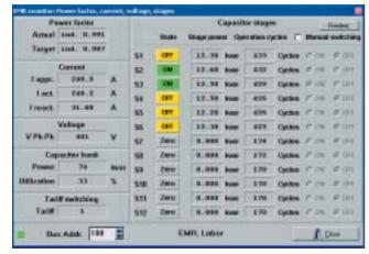
Configuration and remote indication of the measuring values via RS232 interface
