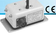
With zero position adjustable to anywhere within the total range of the transducer, voltage output is positive when extending the cable from the selected zero position and is negative when retracting from zero.
