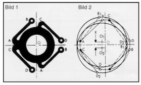
The geometry is made clear in picture 1. The shafts which have to be coupled align. In picture 2, one shaft is staggered x/2 towards the other. Around the same measure have been displaced B1 from B and D2 from D, while the driving arms AB and CD have remained parallel.
