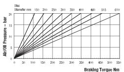
Maximum Pressure 20 bar Maximum Braking Force = 2kN @ 20 bar oil or air pressure Weight of caliper - 0.75kg Volume displacement per 1mm stroke = 3ml
