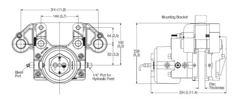
The Twiflex VKCS-FL disc brake caliper comprises a single spring module forming the 'active' side of this floating unit and is available for use where space is limited or to accommodate axial disc float of ±6mm.
