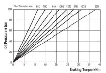
Maximum Pressure 100 bar Maximum Braking Force = 45kN @ 100 bar Weight of caliper - 18.6kg Volume displacement per 1mm stroke at each pad = 15ml
