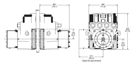
The Twiflex VMS3-SPS disc brake caliper is comprised of two modules bolted to a central mounting plate, 12mm thicker than the brake disc. Minimum disc thickness is 38mm and minimum disc diameter is 1500mm with no maximum except for practical limitations. Based on a development of the earlier Twiflex VMS2-SP disc brake, the VMS3-SPS provides a significant increase in braking force but in a similarly sized package.
