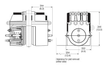
The Twiflex VKHD disc brake caliper is comprised of two halves, or hydraulic modules, and is suitable for use with a minimum disc thickness of 20mm. The modules are mounted each side of a central mounting plate 12mm thicker than the brake disc. Minimum disc diameter is 1000mm.
