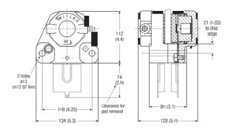
The standard Twiflex T20 disc brake caliper is split caliper design suitable for use with a minimum disc thickness of 12.7mm. Optionally, the caliper may be supplied in a modified form for use with a minimum disc thickness of 8mm. Normally the brake is side mounted, however, for use with a disc thickness greater than 20mm, the split design allows the modules to be mounted each side of a central mounting plate of the same thickness as the brake disc. Minimum disc diameter is 300mm.
