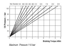
Maximum Braking Force = 20kN @ 110 bar Weight of caliper - 5.82kg Volume displacement per 1mm stroke at each pad = 4.8ml
